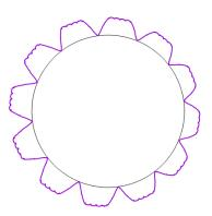
Absolute value of the airgap magnetic flux density, in a machine with eccentricity. The small arigap is to the right.
