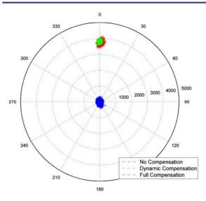
Forces measured between the rotor and an eccentrically placed stator of a smaller generator without any compensation (red), with compensation for rotor defects (green) and full compensation of stator defects (green).
