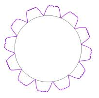
A uniform airgap magnetic flux density that does not produce detrimental forces and losses.
