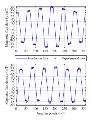
Airgap flux density. The top picture shows the eccentric case (simulated and measured) without magnetic balancing, and the lower picture shows the same with magnetic balancing.
